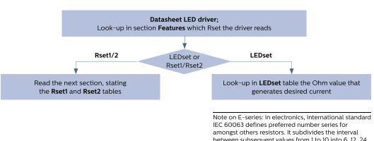
IEC 60063 defines preferred number series for amongst others resistors. It subdivides the interval between subsequent values from 1 to 10 into 6, 12, 24, 48, 96 etc. steps. These subdivisions ensure that when some arbitrary value is replaced with the nearest preferred number, the maximum relative error will be on the order of 20%, 10%, 5%, 1% etc.
